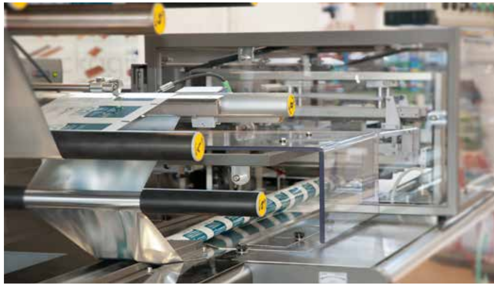
Forming box and longitudinal sealing
