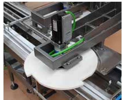
Portioning disk for high speed applications. Up to 400 cycles/min
