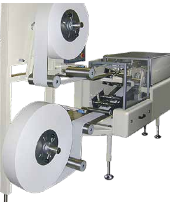
The TPC device in the version with double reel support and automatic film splice system (CAB)
